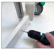
3. Screw the Wall bumper to the cross beam with the self-drilling screws 4 mm
