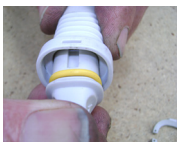
Pic 1. O ring seal
