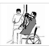
Lower patient (down on hand control) until in desired position. Continue to lower until all straps are slack to remove
